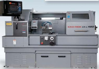
**ProtoTRAK® Lathes** The KING RICH Precision CNC Lathe is the latest generation of Manual / CNC combination lathes, designed with the versatility to handle everything from precision small jobs to heavyduty work. With easy to use conversational programming, this machine can handle many jobs much more efficiently and more accurately than a manual machine can!
